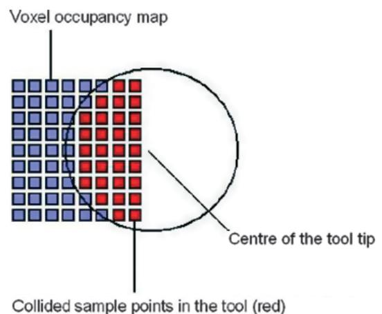
**Figure 1** Volumetric sample points of a tool collide with a tooth model represented by an occupancy map.
